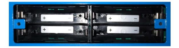
• Lithium-Ion 3.7V button-top rechargeable 18650 Batteries are recommended.
