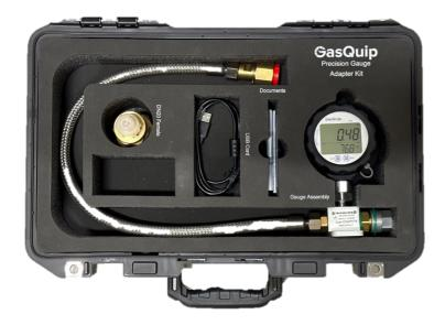
Used to confirm that pressure indicators on an SF6 breaker are accurate anytime gas is moved in or out of the equipment. Utilizes the GasQuip PT5 high accuracy manometer for precise pressure and temperature readings.
